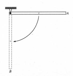
The rod is fixed at one end and allowed to fall from the horizontal position A through the vertical position B.
