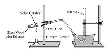
Ethene,  $C_2H_4(g)$  (molar mass 28.1 g/mol), may be prepared by the dehydration of ethanol,  $C_2H_5OH(g)$  (molar mass 46.1 g/mol), using a solid catalyst. A setup for the lab synthesis is shown in the diagram above. The equation for the dehydration reaction is given below.
