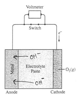
1. Metal-air cells are a relatively new type of portable energy source consisting of a metal anode, an alkaline electrolyte paste that contains water, and a porous cathode membrane that lets in oxygen from the air. A schematic of the cell is shown above. Reduction potentials for the cathode and three possible metal anodes are given in the table below.
