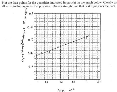
(c) Using the straight line, calculate a dielectric constant for the paper.
