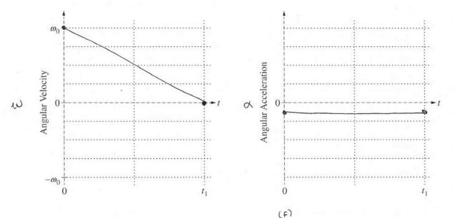
(b) The magnitude of the frictional torque exerted on the disk is  $\tau_0$ . Derive an equation for the rotational inertia *I* of the disk in terms of  $\tau_0$ ,  $\omega_0$ ,  $t_1$ , and physical constants, as appropriate.
