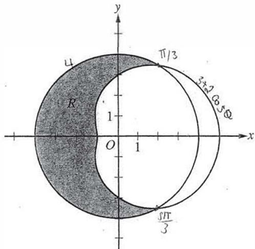
5. GThe graphs of the polar curves  $r = 4$  and  $r = 3 + 2\cos\theta$  are shown in the figure above. The curves intersect at  $\theta = \frac{\pi}{3}$  and  $\theta = \frac{5\pi}{3}$ .
