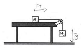
The experiment is now repeated with a modification. The Atwood's machine is now set up so that the block of mass  $M_1$  is on a smooth, horizontal table and the block of mass  $M_2$  is hanging over the side of the table, as shown in the figure above.
