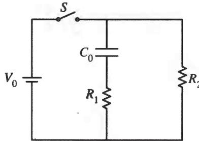
2. In the circuit above, an ideal battery of voltage  $V_0$  is connected to a capacitor with capacitance  $C_0$  and resistors with resistances  $R_1$  and  $R_2$ , with  $R_1 > R_2$ . The switch  $S$  is open, and the capacitor is initially uncharged.
