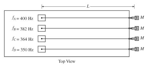
The equation for the velocity v of a wave on a string is  $v = \sqrt{\frac{F_T}{m/L}}$ , where  $F_T$  is the tension of the string and m/L is the mass per unit length (linear mass density) of the string.
