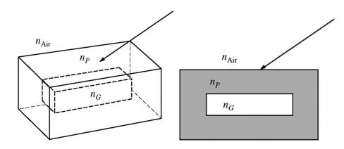
18. Students in a lab group are given a plastic block with a hollow space in the middle, as shown in the figures above. The index of refraction  $n_p$  of the plastic is known. The hollow space is filled with a gas, and the students are asked to collect the data needed to find the index of refraction  $n_G$  of the gas. The arrow represents a light beam that they shine into the plastic. They take the following set of measurements:
