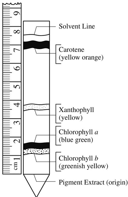
1. Biological molecules can be separated by using chromatographic techniques. The diagram above shows the separation of several spinach leaf pigments by paper chromatography. Using the diagram above
