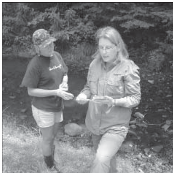
Environmental science teachers Leigh Jenkins (left) of Berkeley Springs, West Virginia, and Cindy Wandling of Charleston, West Virginia, use a CBL probe and handheld calculator to determine the level of dissolved oxygen in a mountain stream.
