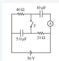
In the circuit illustrated above, switch  $S$  is initially open and the battery has been connected for a long time.
