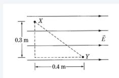
A uniform electric field  $\mathbf{E}$  of magnitude  $6,000 \text{ V/m}$  exists in a region of space as shown above. What is the electric potential difference,  $V_X - V_Y$ , between points  $X$  and  $Y$ ?
